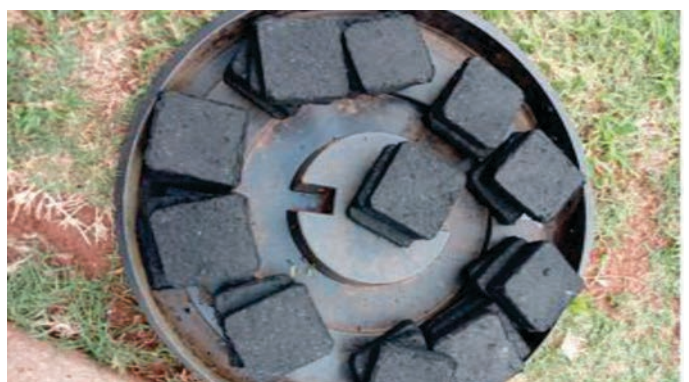
Plates 8 and 9: Briquettes being sun dried
