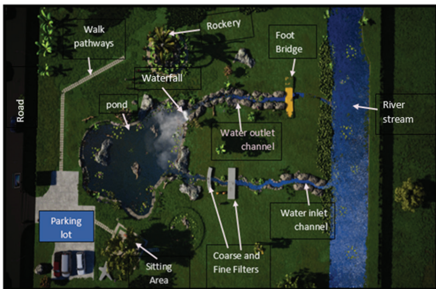
Aerial view of the constructed wetland
